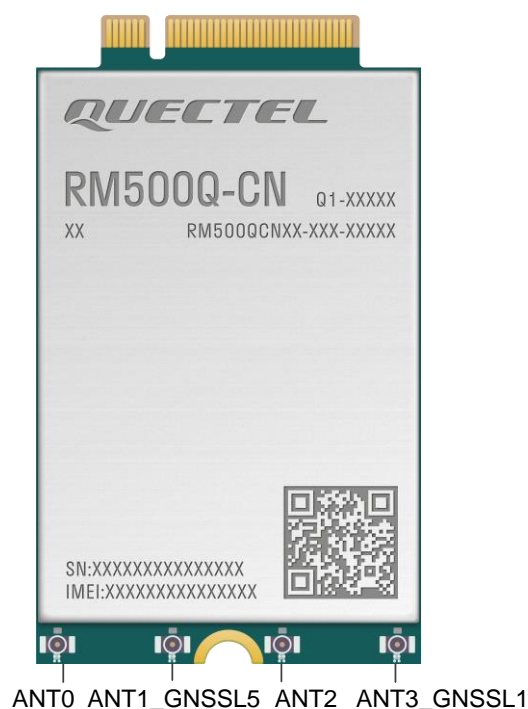
Figure 30: Antenna Connectors on RM500Q-CN
