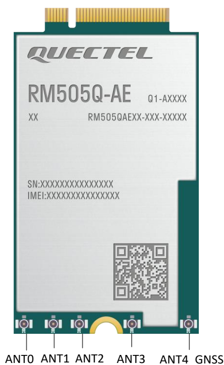
Figure 29: Antenna Connectors on RM505Q-AE
