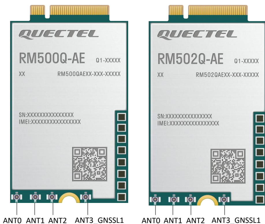
Figure 28: Antenna Connectors on RM500Q-AE & RM502Q-AE
